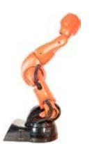
The KR 5 SI was developed differently from most other collaborative robots. Cobots are usually designed by robot manufacturers. But this time, MRK System acts as a robot integrator. They built their collaborative robot concept over a KUKA industrial robot (KR 5 HW ARC)
